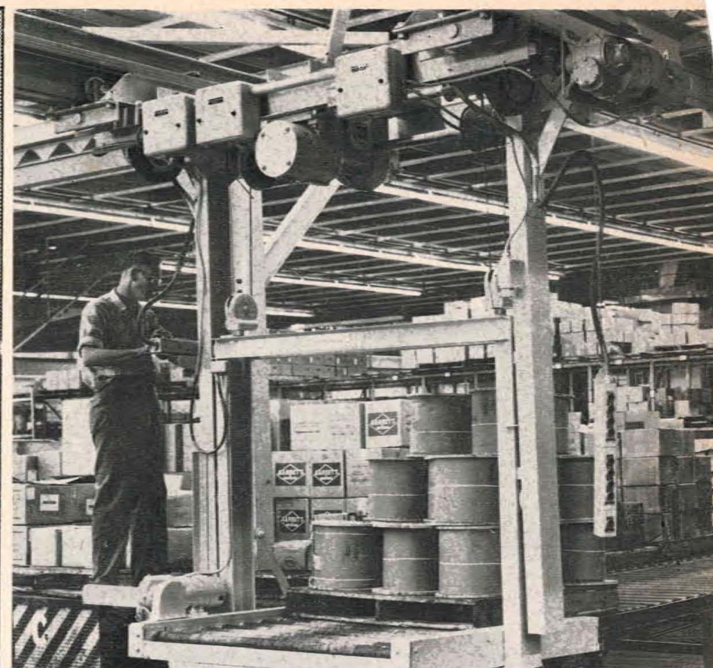
AT ACCUMULATION LINES powered rollers on crane carriage move pallet load onto conveyor. After inspection, materials move to racks, background, or to production lines. All incoming materials clear the receiving dock within 24 hours.
