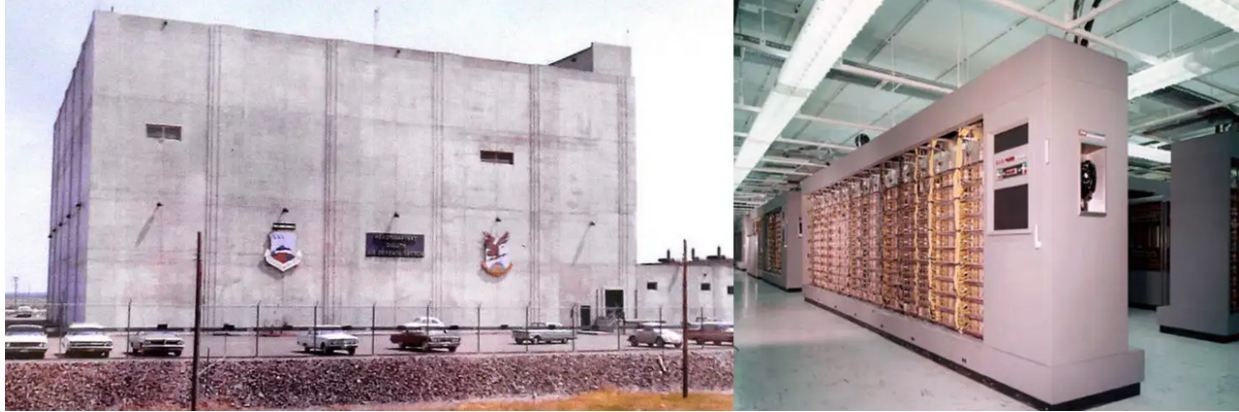
The 23rd Air Division SAGE Building and, right, the AN/FSQ-7 Computer (partial view).
