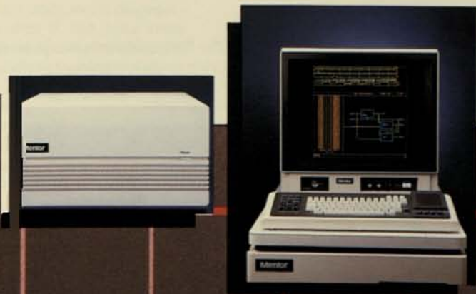
The MIDAS 7000 system gives all the power of a CAE workstation coupled with a high-performance logic analyzer.
