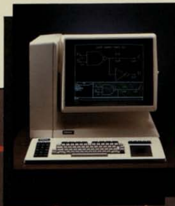
The IDEA 1300 is a cost-effective workstation for schematic entry tasks and includes a 17" high-resolution CRT.
