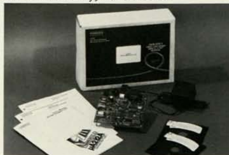
The new \mu A212A Design Kit contains (left to right) User's Manual; Data Sheets and Theory of Operations application note; modem board; and software.
