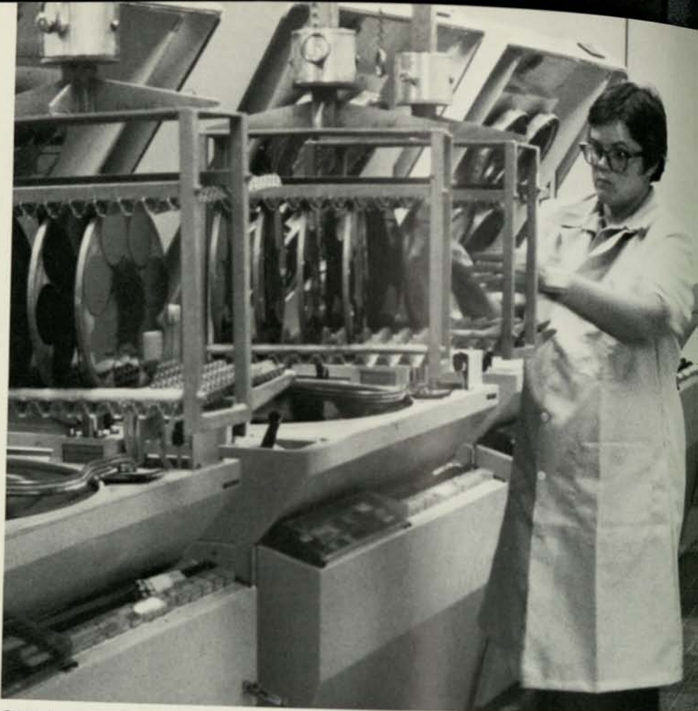
Carol Armstrong loads wafers nearing completion into large polishers. Wafers are mounted on round metal plates with heated wax in preparation for polishing.
