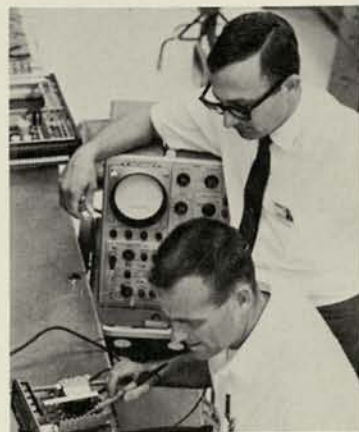
Jack Vossler, left, Associate Engineer, checks out engineering prototype of the Model 8050 he is constructing. Jack, assisted by John Dour, uses an oscilloscope to monitor circuit operation of the counter.
