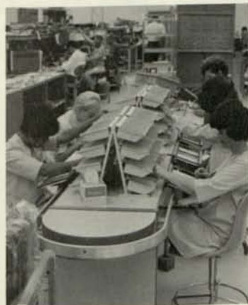
Mass production takes place at assembly line "roundabout." Printed circuit boards attached to an endless belt move between loading stations where electronic assemblers insert pre-formed components into plated-through holes. "Stuffed" boards are removed and dip-soldered at another location.
