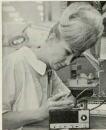
After approval of the engineering prototypes, a small number of meters are produced for sales evaluation and manufacturing studies. Here, Carean Bigner, Chassis Wirer, is assembling a pre-production Model 8050 in the Instrumentation Model Shop.
