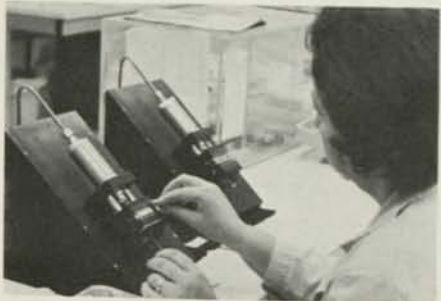
Helen Silva straightens leads on devices prior to the actual packing process. Approximately 1000 units can be straightened per hour.
