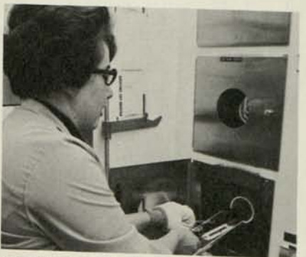
Loading the diffusion furnace with a run of wafers is Judy Nelson.
