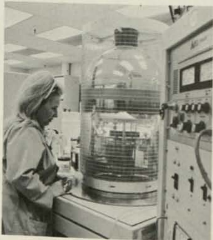
Millie Baumier is adding the aluminum on wafers by using an evaporation machine.
