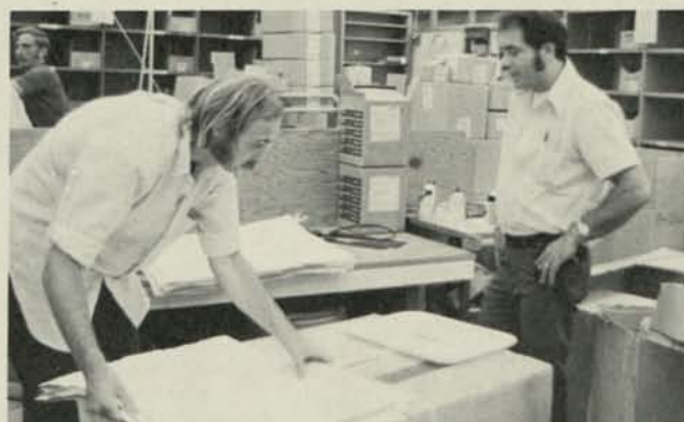
Oliver Connelly (left) and Frank Varano inspect government bags for return to vendor by pulling them over their heads to check for holes. They are considered "rejects" if a hole is found.
