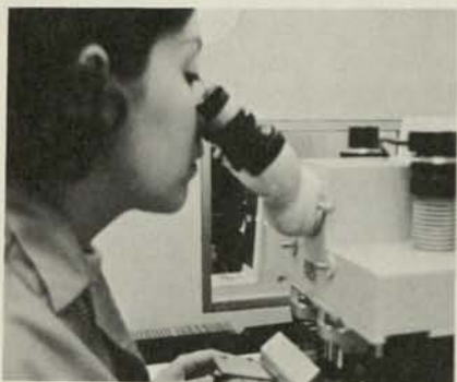
Sarah Valenzuela is exposing, aligning, and designing a pattern on the wafer before it goes to final checking.
