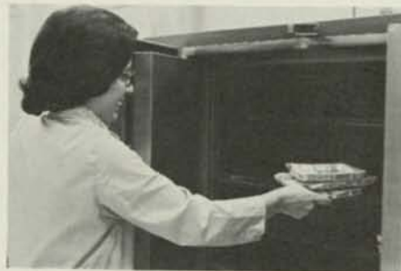
Charlene McDonald, assembly work leader, places units in 302°F oven for half an hour to dry the markings before final electrical test.
