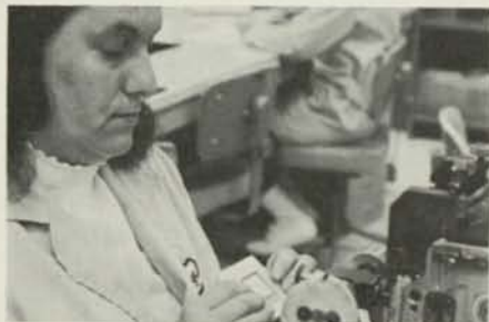
Olga Chribas marks devices in a 64 Lead Flat Package which is done on a special marking machine. An operator can mark up to 2100 units a day.
