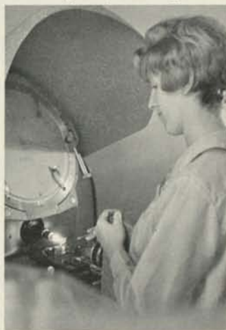
Machinist Marlene Crosby measures a bonding tool she just completed lapping. She's using an optical comparator.
