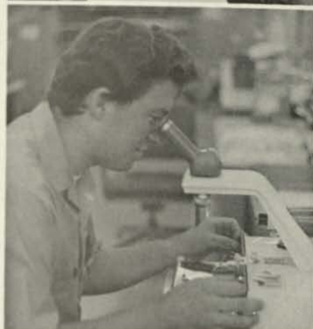
Juan Moraida adjusts and cleans the needle on EMB Wire Bonder in Metal Can area.
