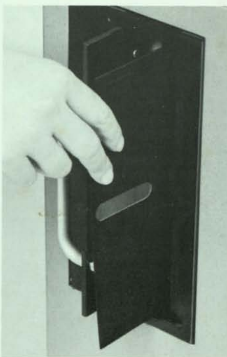
Replaceable memory discs store up to 50,000 words each.
