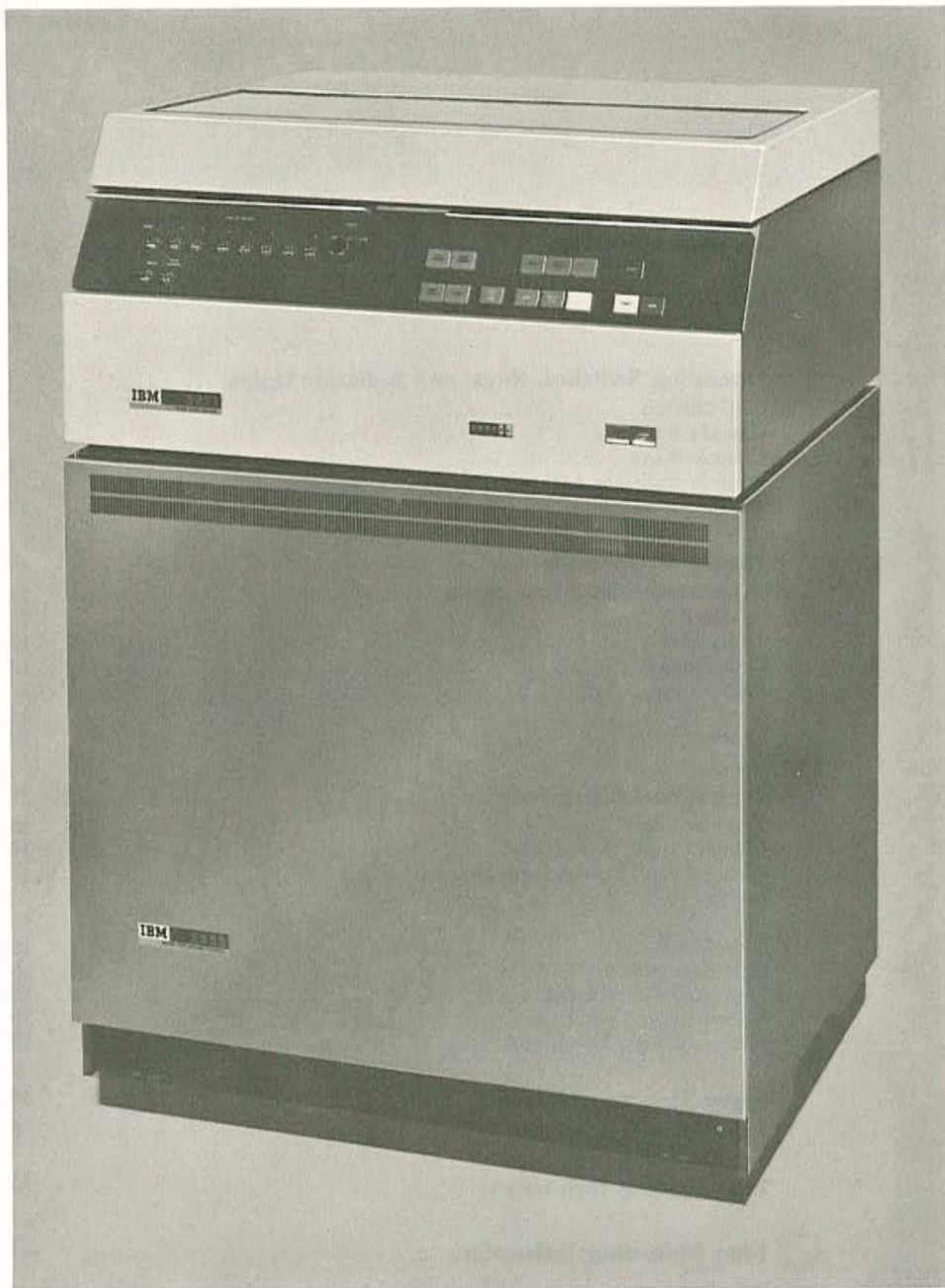
Figure 1. IBM 2671 Paper Tape Reader and IBM 2822 Control Unit
