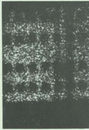
FIGURE 13 Ion Probe Mass Analyzer Scanning Images — Silicon Semiconductor (150X)
