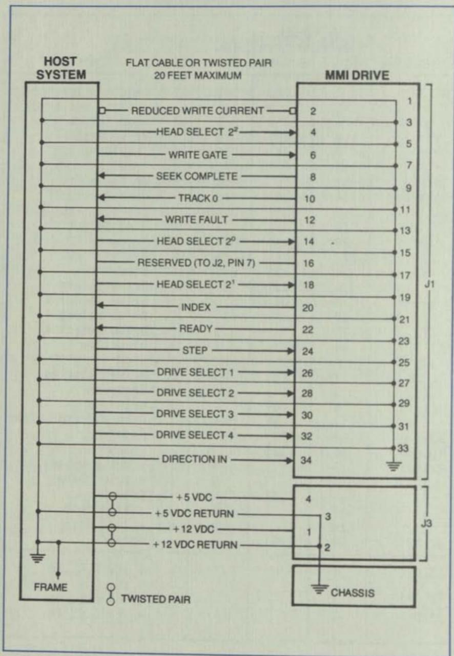
Figure 9. J1/P1 Control Signal Cabling
