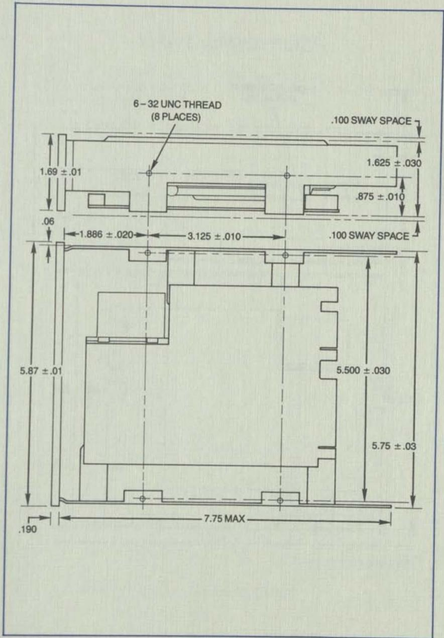
Figure 3. M212/M225 Mounting Dimensions
