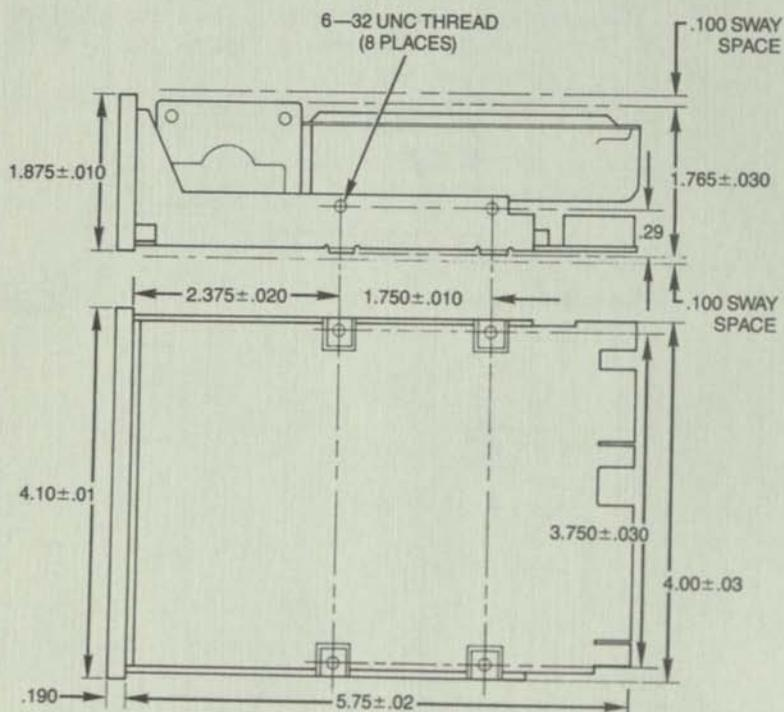
Figure 2. M125 Mounting Dimensions
