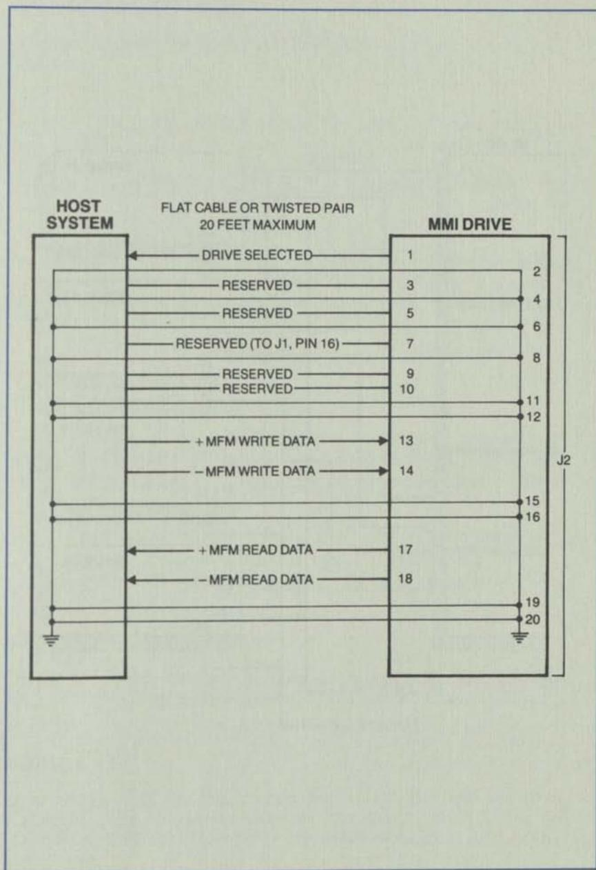
Figure 10. J2/P2 Data Signal Cabling
