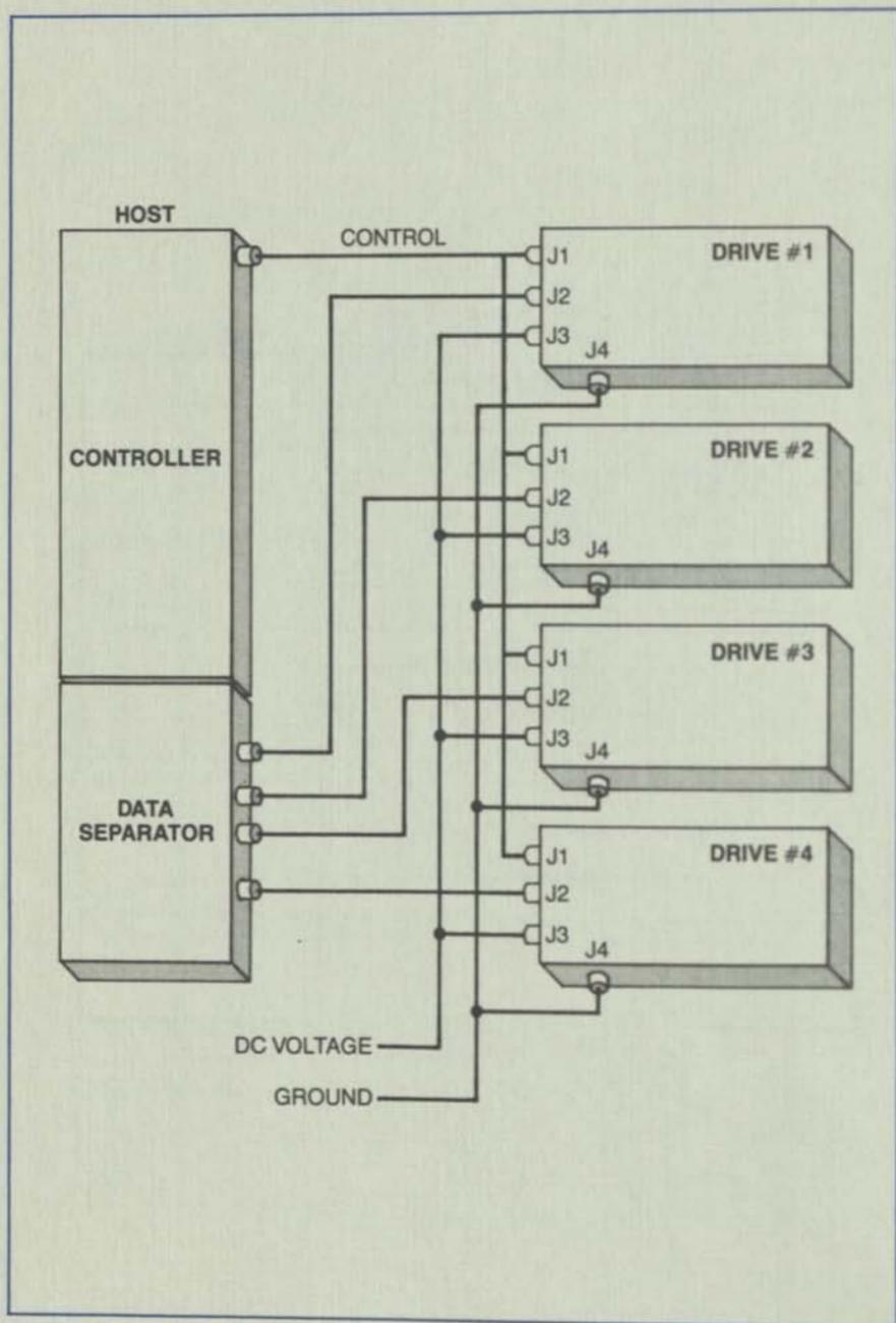
Figure 11. Cabling for Four-Drive System
