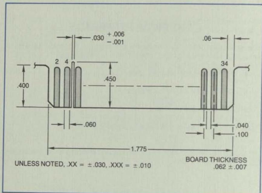
Figure 6. J1 Connector Dimensions
