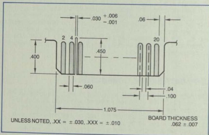
Figure 7. J2 Connector Dimensions
