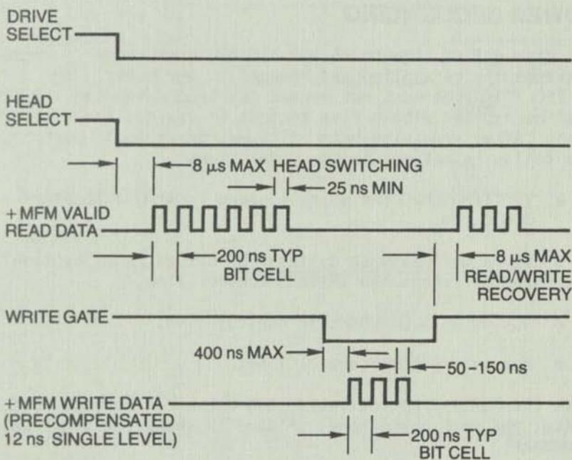
Figure 18. Read/Write Data Timing
