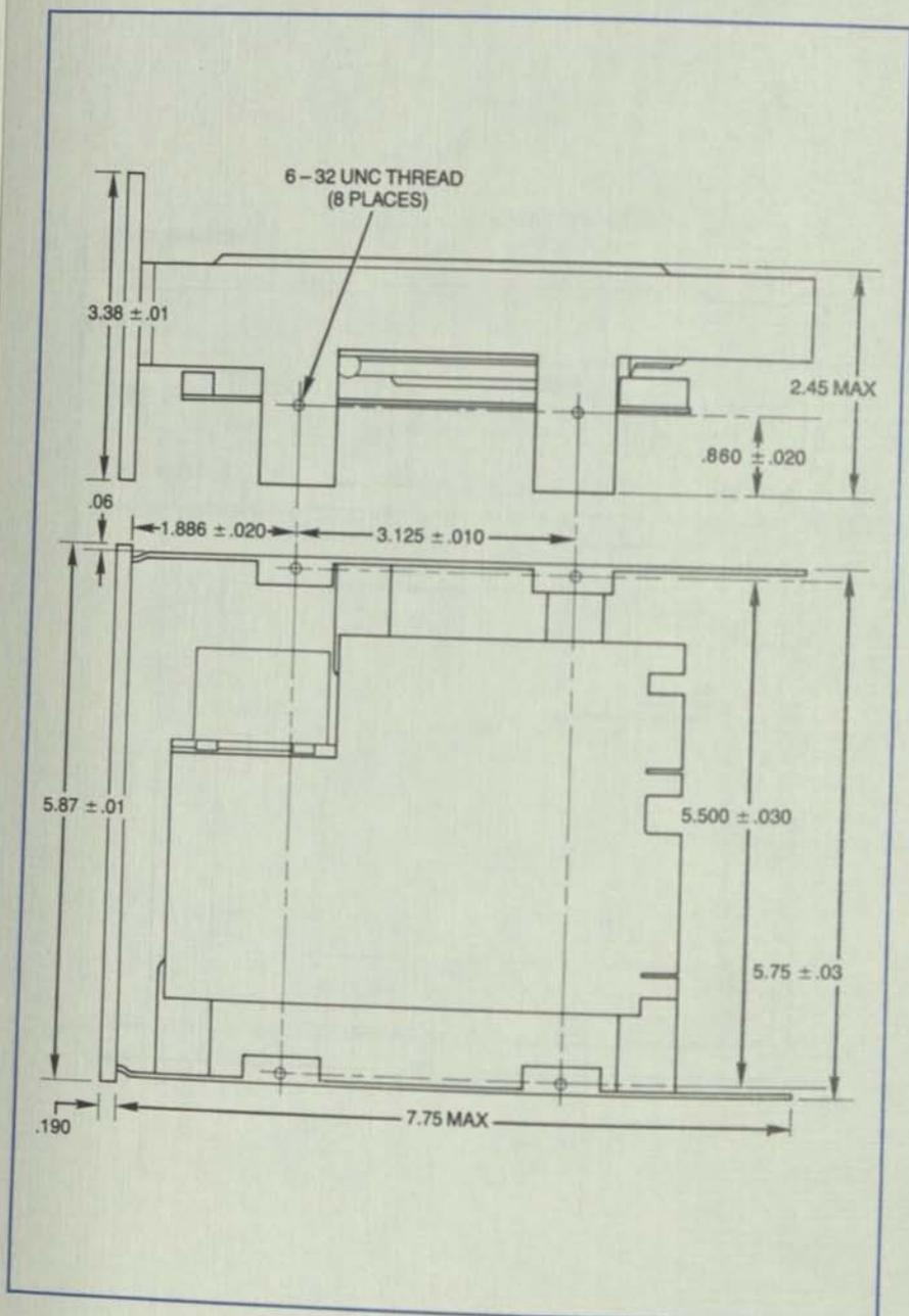
Figure 4. M312/M325 Mounting Dimensions
