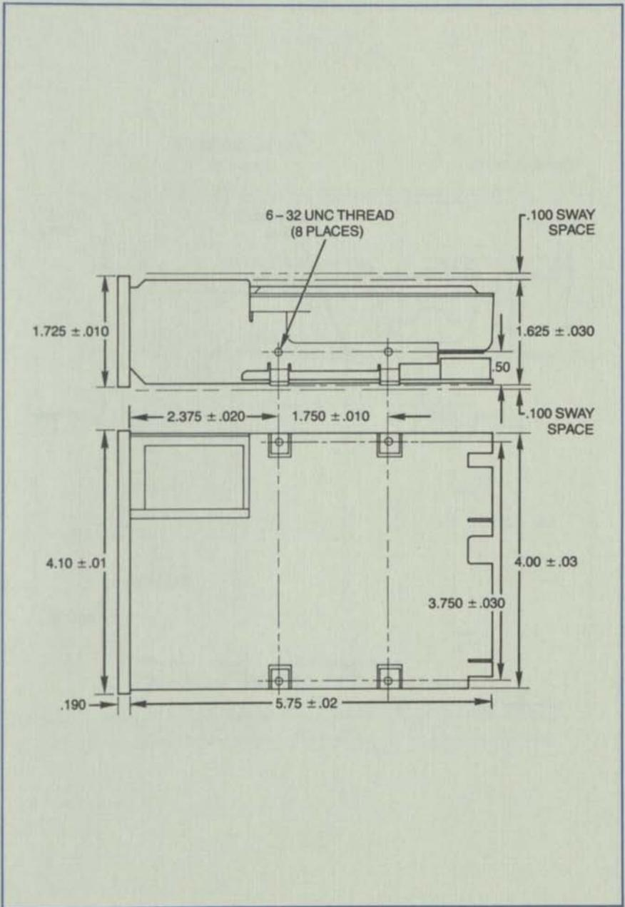
Figure 1. M12 Mounting Dimensions
