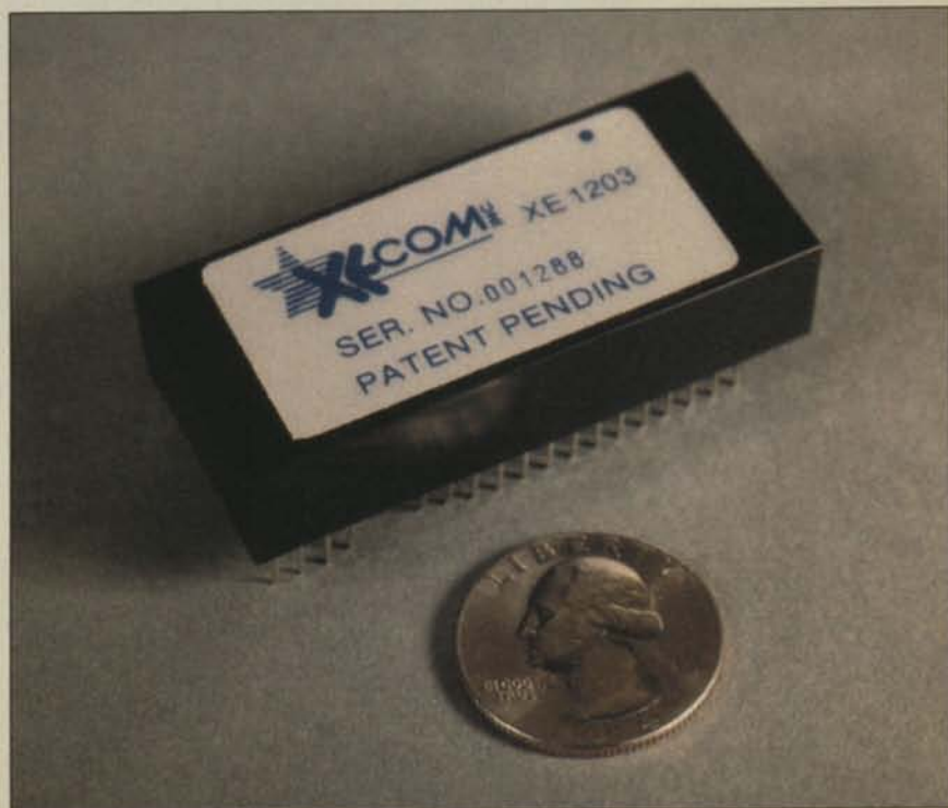
Photo 1: A close-up of the MOSART module as a 1200-bps modem (and more) on a chip.
