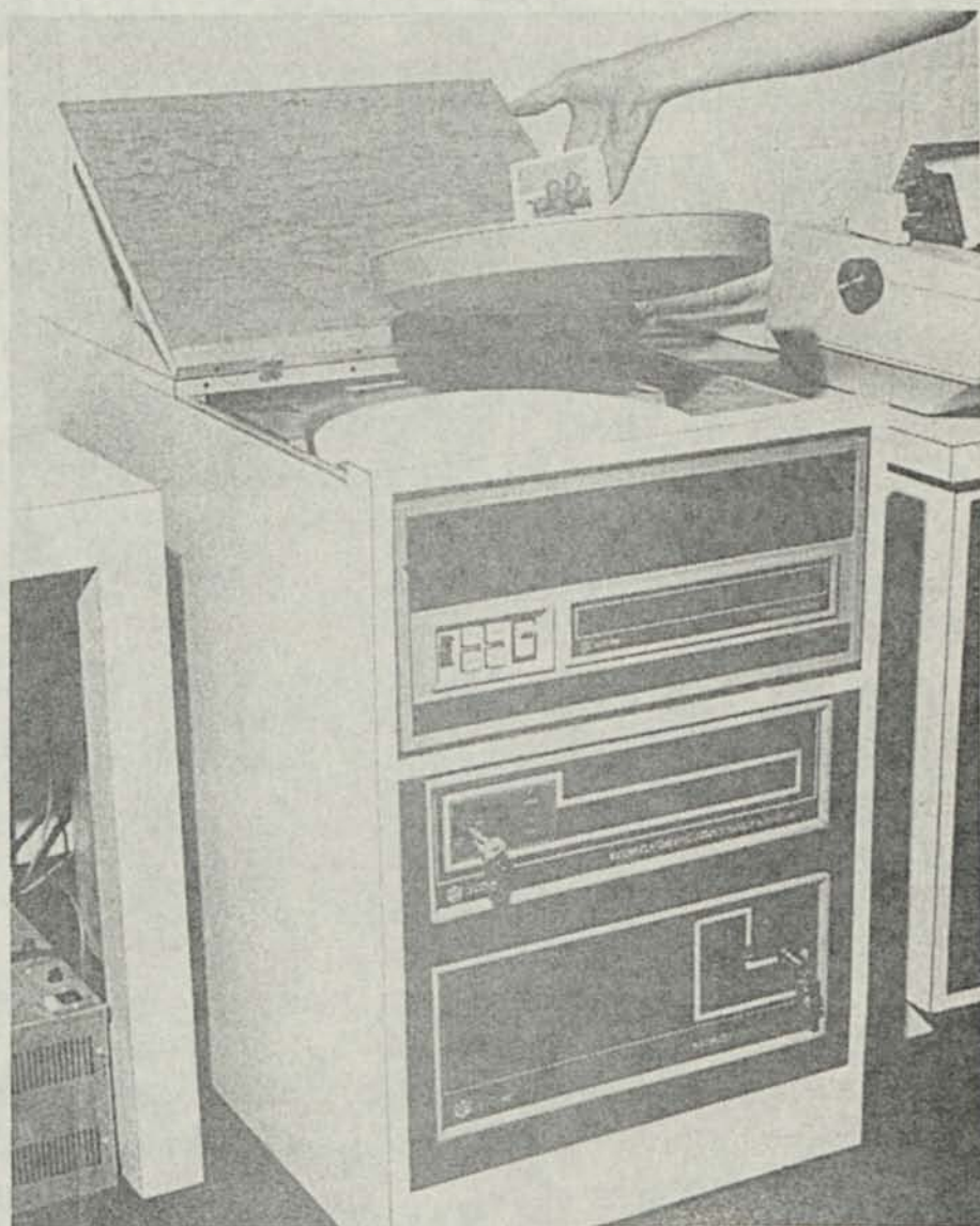
Figure 8-5. The Altair hard disk drive and controller with the Altair 8800b Turnkey microcomputer.
