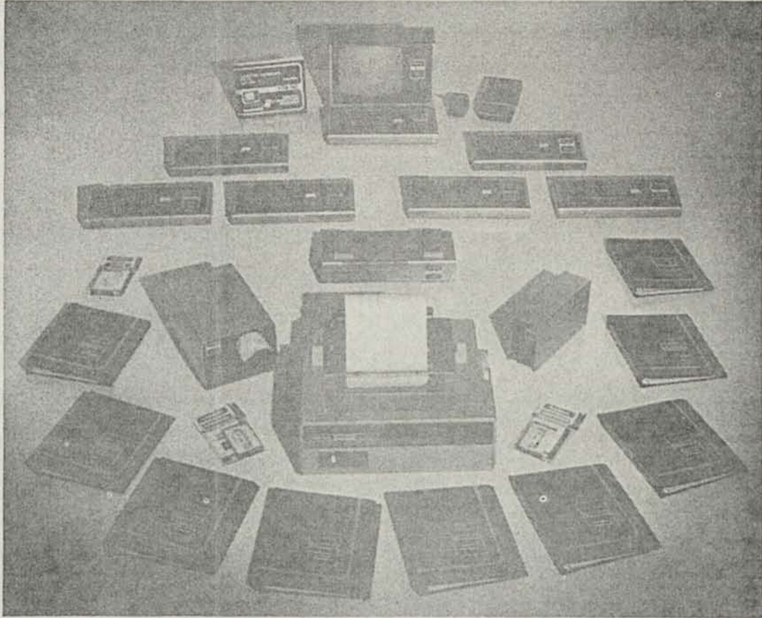
Figure 6-5. The TRS-80 microcomputer, peripherals, and software. The basic TRS-80 microcomputer is shown in the rear. In front of it are other keyboard/microcomputer units to symbolize the available options. In the center is the TRS-80 line printer, and slightly behind it is the TRS-80 expansion interface. To the right is the TRS-80 Mini-Disk system, and to the left is the TRS-80 screen printer. In the foreground are binders containing TRS-80 software.
