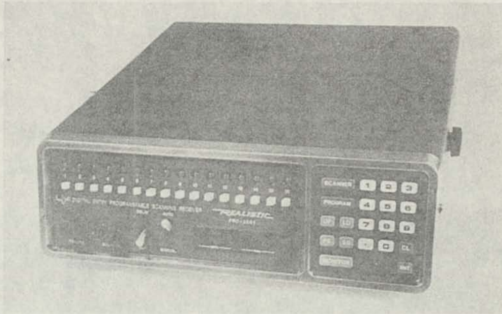
Figure I-5. Radio Shack's PRO-2001 UHF/VHF Communications Scanner. This device is programmable and receives 6 bands. Frequencies being scanned, monitored, or programmed into its memory are displayed on a digital readout on the front panel.
