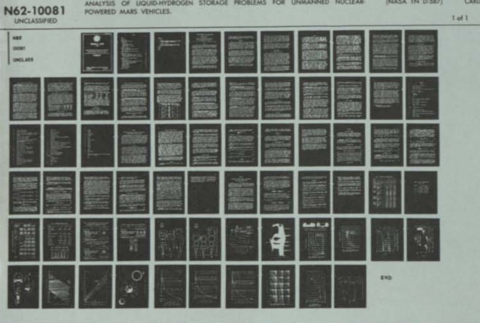
SAMPLE of 5-by 8-inch microfilm sheet used by NASA. It can hold up to 82 pages of 8½-by 11-inch size. Identifying tab at top is visible without enlargement.
