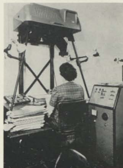
DOCUMENTS being filmed by step and repeat camera. Console at right of operator gives control over negative.
