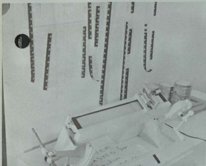
CUSTOM-BUILT slitter for cutting away excess from 35mm microfilm during the preparation of the microfilm card which will allow mailing of an 80-page document on one sheet.
