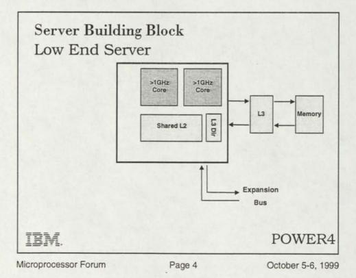
Power4: A Dual-CPU Processor Chip Server Building Block
