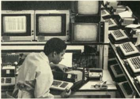
As part of a quality control procedure that begins during assembly and ends at the dealer destination, assembler Vincent MacShate monitors video and sound functions of an Apple III.
