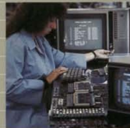
In an Apple III test sequence, assembler Maria Mathis monitors video and sound functions.
