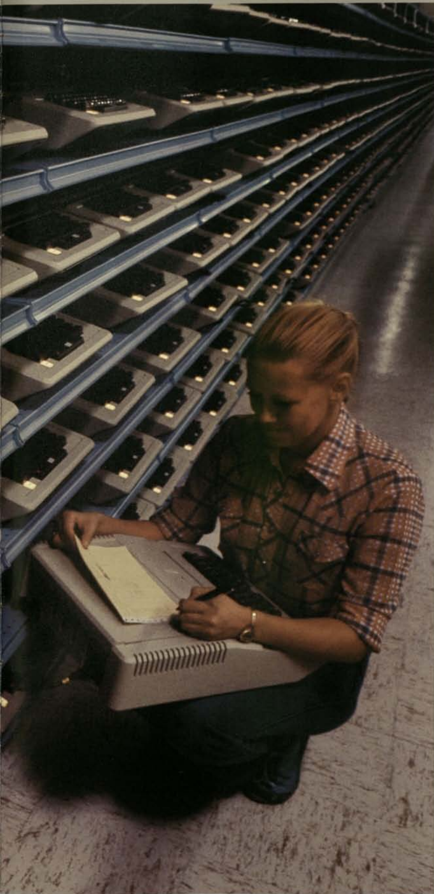
Volume production requires high-capacity quality control and test capability. At left, material processor Susan Walker readies an Apple II for a four-day testing procedure.
