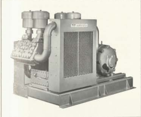
base-mounted multi-v-belt driven compressor (M-125 illustrated, with belt guard)
