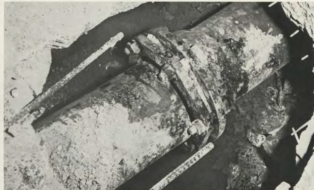
With a portion of the floor chipped away, this is the separated mechanical joint. The two rods in the picture are merely a part of the concrete reinforcement. When the detector check valve (see picture left) shifted, it obviously caused this joint to pull apart. In order to check out the rest of the line, it was necessary to chip away floor the entire length of the pipe. This eight inch cast iron fire water supply line had withstood a test of 200 pounds per square inch for two hours as specified. The break occurred after the building was occupied.
