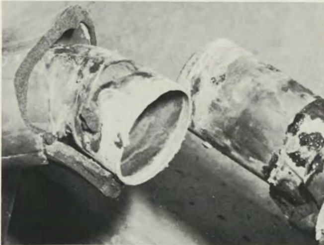
Photograph taken of a break in a 2½ inch copper secondary chill-hot water return line before the components were removed. The separation occurred at a 45° angle joint in the ceiling-hung pipe. Examination showed that the pipe was irregularly inserted into the filling socket and the solder interface was also irregular with a portion of the circumference sub-standard. The results of the investigation indicated that the pipe was not assembled in a workmanlike manner.
