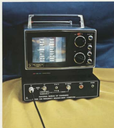
Figure 8. Prototype of a digital offset computer.
