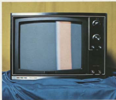
Figure 7. Prototype of a color bar comparator.
