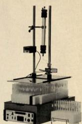
Effluent peaks between recorded event marks aren't always deposited in the indicated test tube. Event marks locate tube changes, but the adjacent curve monitors the effluent as it is passing through the flow cell, not into the tubes. The resulting discrepancy can be quite large if the effluent tubing, flow rate, and collected sample size are not perfect. Manual chart corrections are inaccurate and time consuming.
