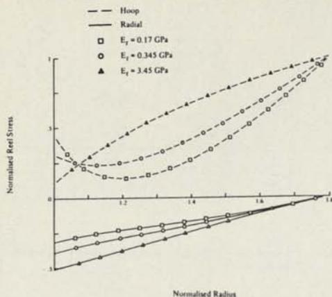
Fig. 8—Predicted effect on the tape's circumferential and radial stresses of the tape's radial modulus.
