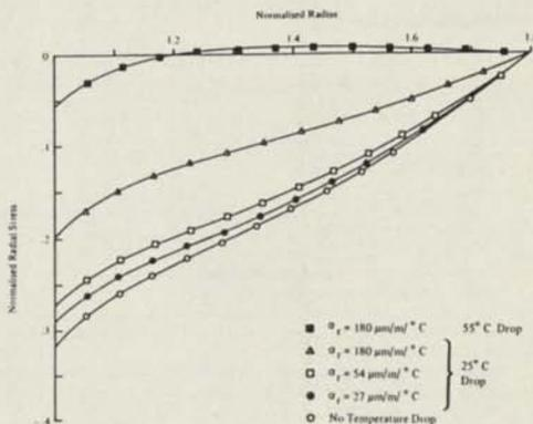
Fig. 10—Predicted effect on the tape's radial stress of a temperature drop of (a)  $25^\circ\text{C}$  for various tape radial coefficients of thermal expansion, and (b)  $55^\circ\text{C}$  for tape radial coefficient of thermal expansion  $\alpha_r = 180 \mu\text{m/m}^\circ\text{C}$ .
