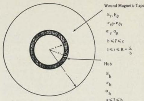
Fig. 2—Fully wound tape geometry
