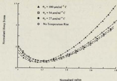
Fig. 9—Predicted effect on the tape's circumferential stress of a temperature rise of  $25^\circ\text{C}$  for various tape radial coefficients of thermal expansion.
