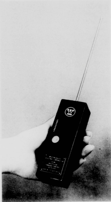
This 30-megacycle command control receiver, also built with integrated circuits, contains a high percentage of linear and digital circuit blocks. The interior of this tiny receiver is shown below.
