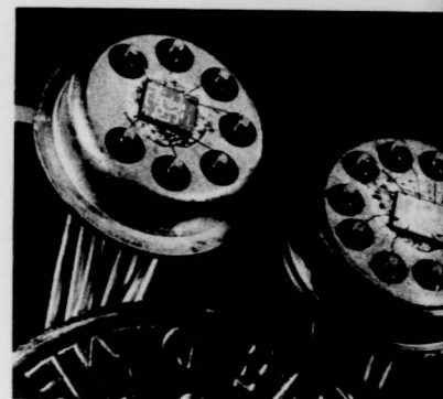
Norden integrated circuits in equipment for Polaris submarines are expected to be nine times more reliable than previous conventional components. Left is an input buffer. Right is a low noise preamplifier. The units were designed for the Ships' Inertial Navigation System (SINS) equipment.
