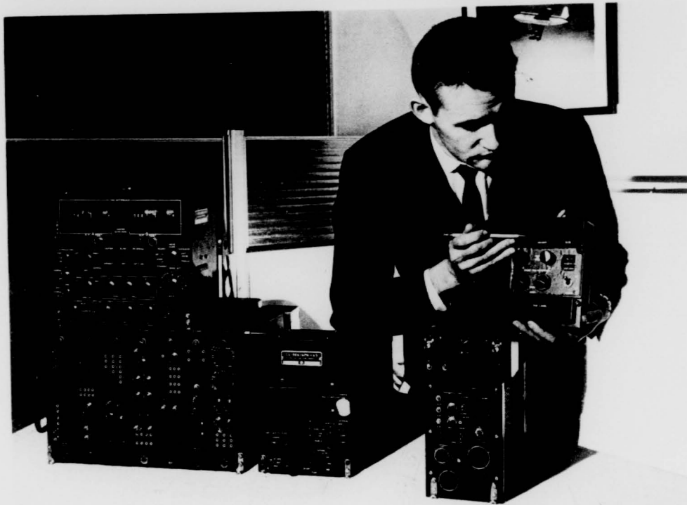
The integrated circuit Loran-C receiver on the right in comparison to the conventional Loran-C receiver on the left is three times more reliable, requires much less power, and is far simpler to use. The Air Force will use the improved receiver aboard the Apollo recovery aircraft, HC-130M.
