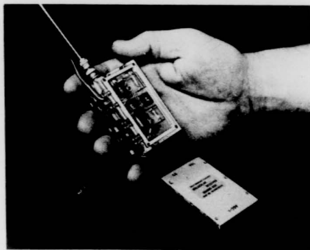
The AN/ARC-63 communications receiver was the first non-digital equipment to make extensive use of integrated circuits—with a resulting 35 to 1 reduction in size and weight over a comparable transistor version of the same receiver.
