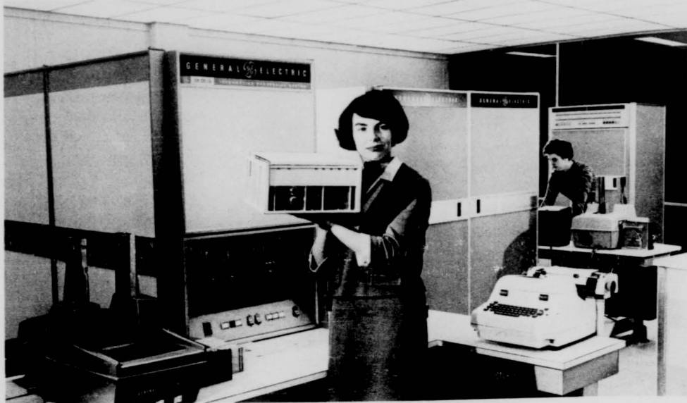
General Electric's 18 lb., Model A-212 aerospace-oriented integrated circuit computer is shown here. In the cabinets in the background is a GE Model 225 general purpose computer using transistor circuits. The A-212 requires only 67 watts for operation.
