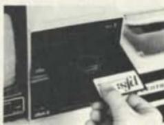
with the label upwards, as shown. The oval cutout in the diskette jacket should enter the drive first. The label should enter the drive last. Gently push the diskette until it is entirely inside the drive. Then close the drive door by pushing it down.
