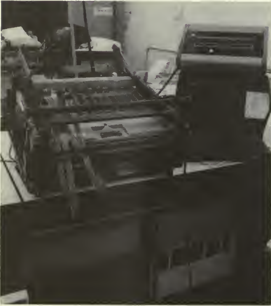
Figure 26. GenRad Corp. (GR) tester for modules.
