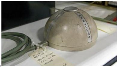
full revolution of the encoders between data words which meant ambiguous code values. The computer had to recognize and correct that to keep the cursor from jumping on the screen.
