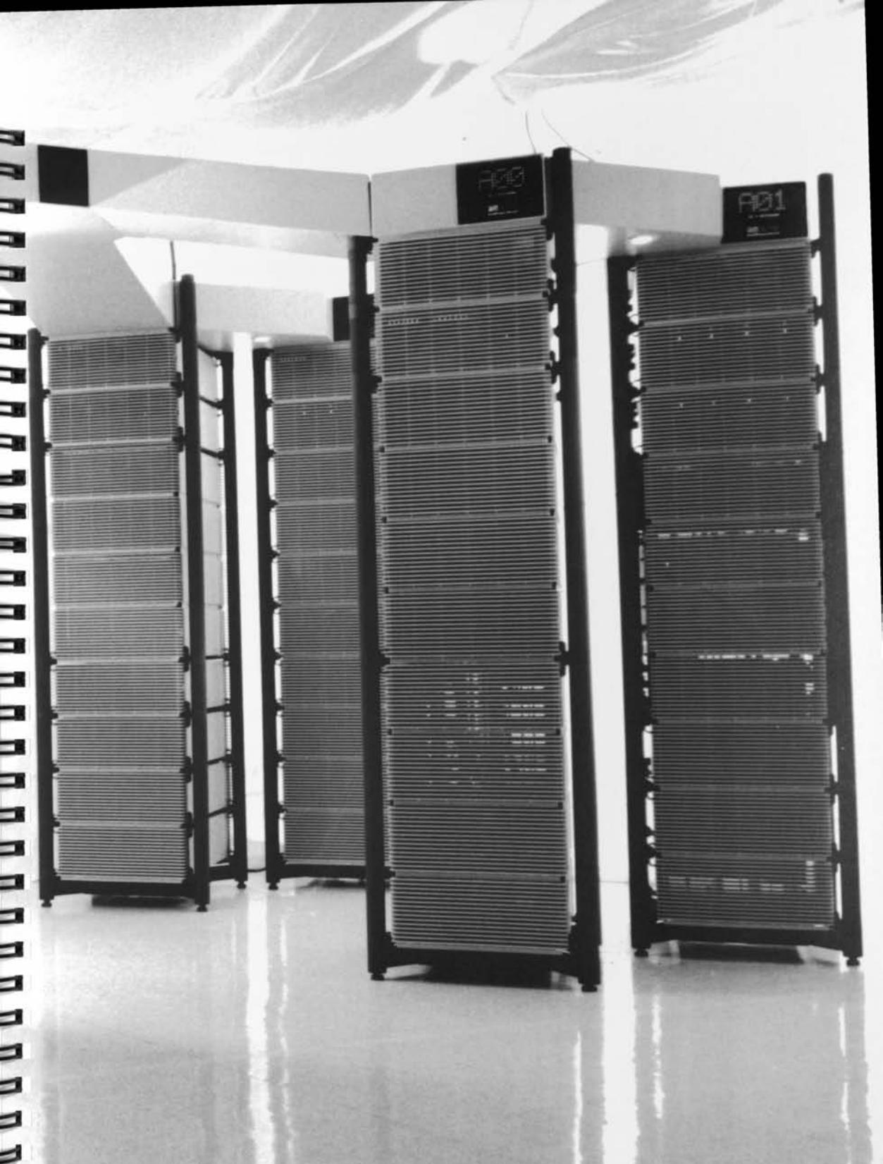
CENTER SPREAD: THIS KSRI-256 IS A MULTI-TOWER COMPUTER CONFIGURED WITH 256 PROCESSORS PROVIDING, 10,240 PEAK MFLOPS, 8,192 MBYTES OF MEMORY, A MAXIMUM DISK CAPACITY OF 3,600 GBYTES AND 3,600 MBYTES/SEC. OF I/O CAPACITY. THE TOWER GROUPS ARE CONNECTED BY A CABLE TRAY WHICH CONTAINS THE INTERSYSTEM NETWORKING AND ELECTRICAL WIRING. NO SPECIAL COOLING OR FLOORING ARE REQUIRED.
