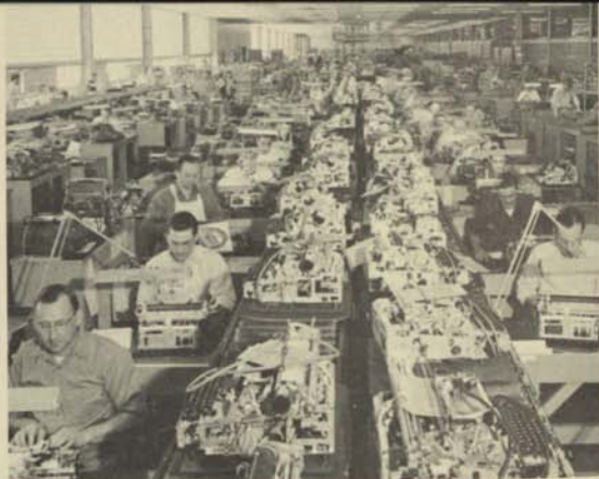
On this assembly line, more than 2400 parts are put together to complete each IBM electric typewriter.
