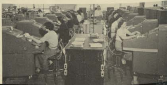
On this assembly line, more than 2400 parts are put together to complete each IBM electric typewriter.
