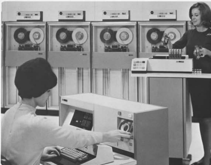
▲ The IBM 129 Card Data Recorder has a monolithic-circuit memory that helps speed punching of familiar 80-column cards for computers and other business machines.
