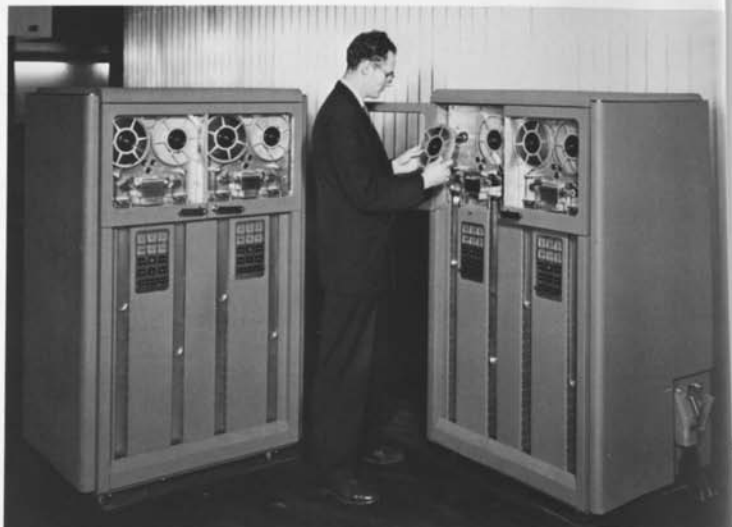
▲ A demonstration of tape reel removal. The vacuum columns clearly show the long tape stress during reel reversal.
