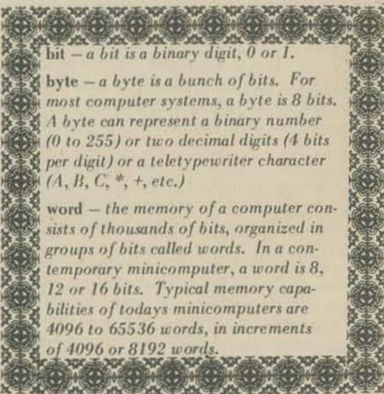
For the average school BASIC user all this doesn't mean a hill of beans. Word length is invisible to the BASIC user so whether you're using an 8 bit, 12 bit or 16 bit machine makes no difference. Is it obvious that 4096, 16 bit words is more memory than 4096, 12 bit words or 4096, 8 bit words? (We think so.)
