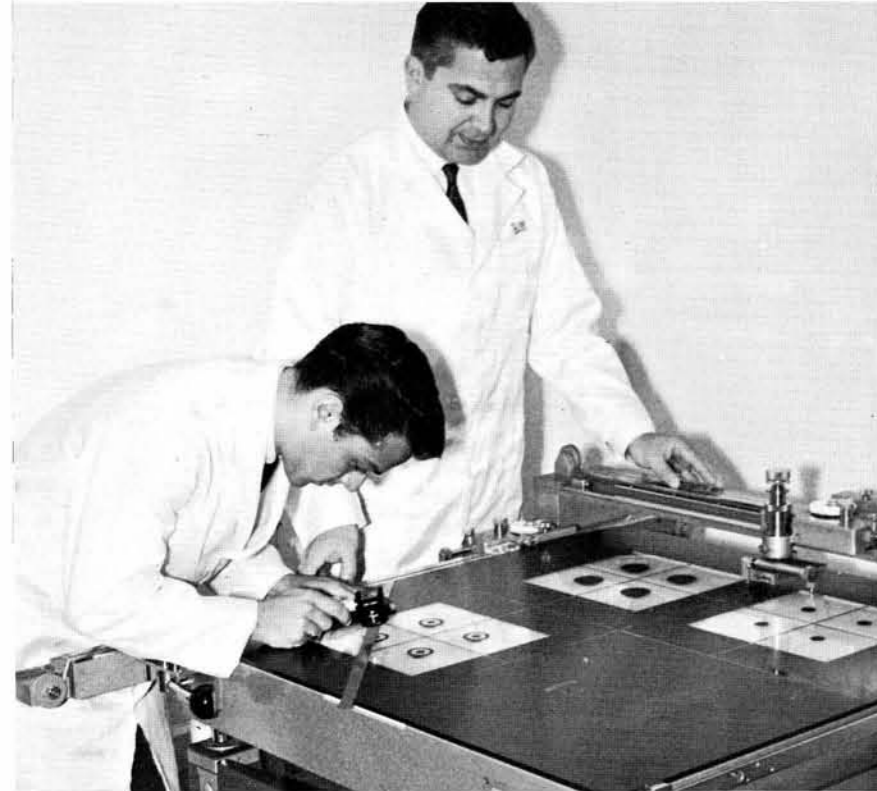
Vince Fulginiti, Lab Technician, bending, and Bill Duff, Photographic Specialist, check measurements of a newly drawn pattern on the Mask Manufacturing Lab's new coordinatograph. A razor-sharp blade on the precision-built instrument cuts patterns in black paper stretched over glass in the first step of the mask-making process. Since his work must be accurate to a hairline, Vince checks the patterns with a precision magnifier.
