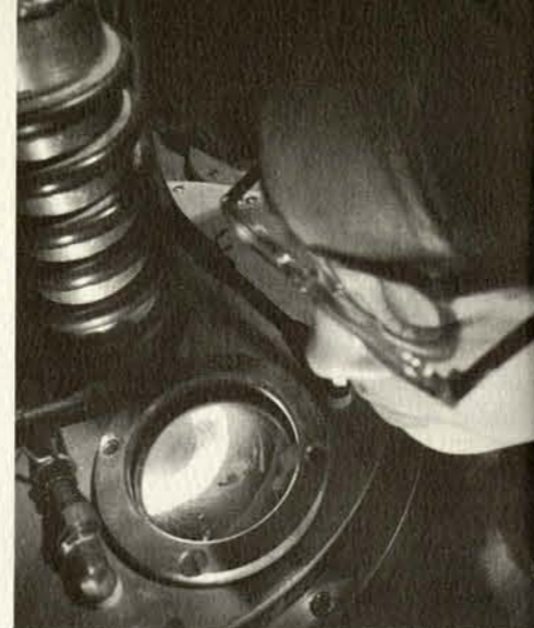
Technician checking progress of a crystal of pure silicon, being prepared by the Czochralsky method. Chunks of silicon are placed in a heatproof container and melted in an oxygen-free atmosphere. Then a tiny "seed" crystal is touched to the surface of the molten silicon and slowly withdrawn from the container. The molten silicon atoms arrange themselves on the seed in a precise pattern called a "single crystal", and eventually all the molten silicon is transformed into a long, cylindrical ingot for later processing and slicing.
