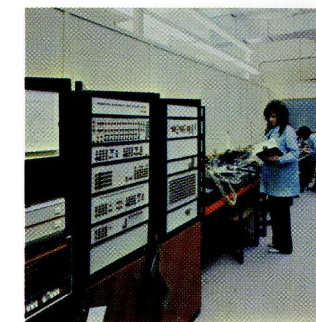
These MOS 8192-bit read-only memories, still in wafer form, are being automatically tested. Upon completion they will be used in computerized reservation equipment, such as airline ticket counter terminals.
