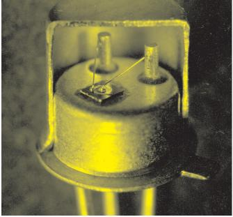
recalled in a recent telephone interview. On 2 March, Hoerni wrote another entry in his notebook titled "A method of manufacture of PNP transistors with oxide protected junctions." In two more pages of text and drawings, he indicated specifically how to fabricate such a device, though still stubbornly using silver for the electrical contacts on the top side. By then, his technicians were already transforming his novel ideas into actual fabrication processes.
