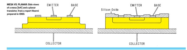
closer to that of the mesa, with contacts on both sides of the wafer. In Noyce's much more famous patent, "Semiconductor Device and Lead Structure," filed three months later, the single-side feature is a fundamental aspect of his planar integrated-circuit structure. But neither man's lab notebook mentions the idea—suggesting that it probably emerged from the fertile give-and-take discussions that spring and was later added to the patent applications.
