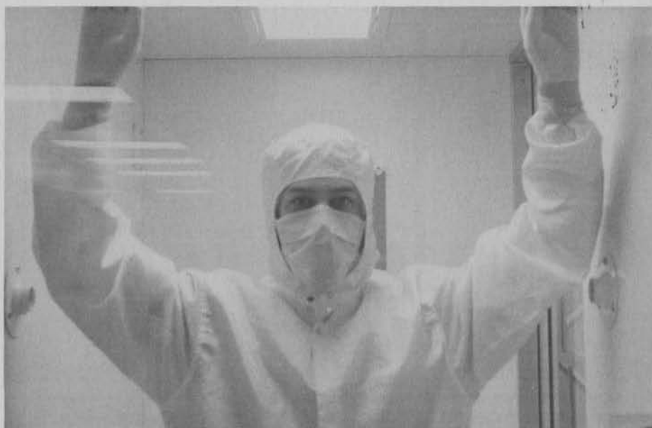
Mike Wageman , head disk assembly lead operator in LDDD, works in his "bunny suit" much the same way a surgeon operates in his scrub gown. Before entering the clean room, Wageman takes an air shower.
