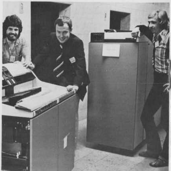
Rolling a 3670 into Folksam are FE Torgny Bengtsson and Sales Rep Bernt Ohlen. FE Karl-Ake Jonsson stands ready with a 3672 control unit.
