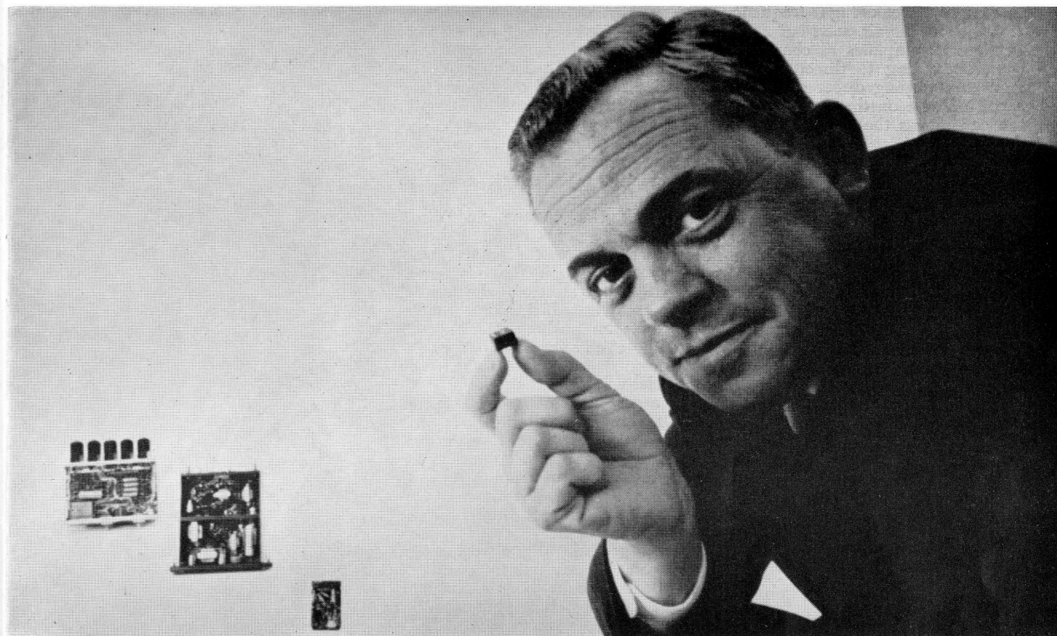
Amplifier shrinks from tubes (left) to transistors to microminiature to integrated circuit held by Lear's David Moore
