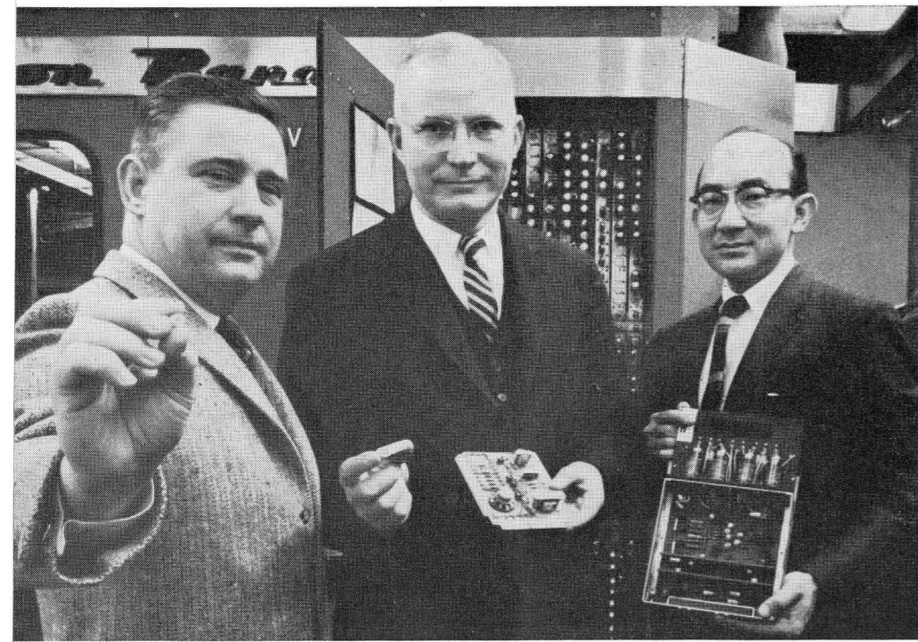
Progressive shrinkage in computer circuits: From right, Chuan Chu, Univac Div., holds electron tube module; Burke H. Horton, Univac, a transistorized version and a subminiaturized digital device for an airborne computer now in production; and W. R. Sittner, Sperry Semiconductor, a tiny integrated semiconductor circuit.
