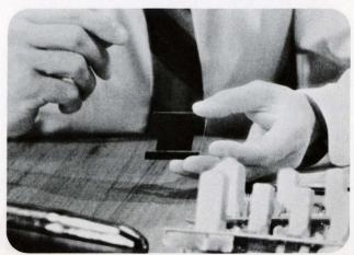
Now the artwork, which I showed, was only one potential mask. Here is the artwork, in reduced plastic overlay version, of a complete set needed to make an integrated circuit. There are five to seven or even more of these potential masks. All of these must align carefully and precisely.
