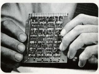
Now integrated circuits can be used not only for digital but also for linear circuits. Here is an i.f. strip. It's transistorized and hence perhaps three years old. Here is its integrated circuit counterpart, providing exactly the same function. Notice how much simpler it is. The wiring is roughly the same, the simplicity is greater. Hence, we can expect that it will not only be cheaper, but more reliable, and these are perhaps the most important contributions of integrated circuits.
