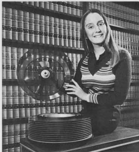
The new Mark XI Disc Pack, shown here, is capable of storing up to 200-million bytes of data, equivalent to the number of words contained in approximately 2,500 standard sized novels.
