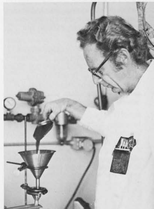
Senior Chemical Technician Rich Kruger uses jet mill to produce new all-purpose duplicating toner.
