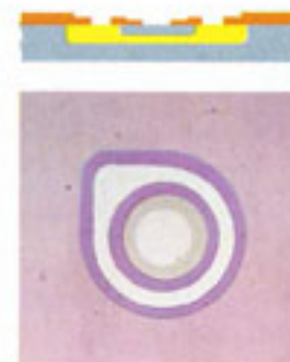
Base and emitter contact areas are etched through the oxide coatings. Precision masking keeps etching well away from junctions. Protective oxide over junctions remains undisturbed.
