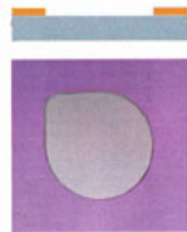
A window is etched through the oxide to prepare for base diffusion. Surrounding oxide has been masked against etching by a photo lithographic technique.
