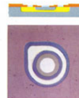
Metallizing of base and emitter contacts completes the processing of the wafer prior to separation into individual dice. At no step have the junctions been exposed to contamination.
