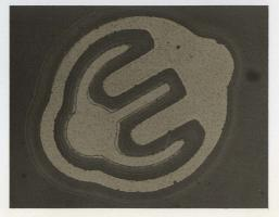
Micrologic: Within a year after introducing the Planar process, Fairchild produced the first practical microcircuit—integrating transistors and resistors, plus all the necessary interconnections, in a single, monolithic chip of silicon. A full spectrum of highly developed semiconductor skills was utilized: precision optics and mask-making; the Planar diffusion process; metal-over-oxide; mounting and lead bonding; testing and test equipment design and production.
