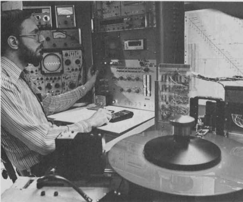
As part of the quality assurance procedure, the heads performing the read/write function in disc drives are tested to assure proper electrical performance through this automated machine, which is controlled by a microprocessor and displays the test data visually through an oscilloscope.
