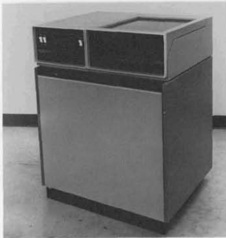
660 Disc File , with 30-megabyte capacity, is a low cost, high speed information storage system.
