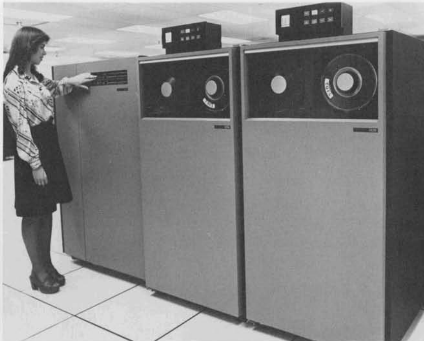
Advanced 6250-bpi tape drive, providing superior performance and cost-effectiveness, is a major addition to the Memorex line of storage products.
