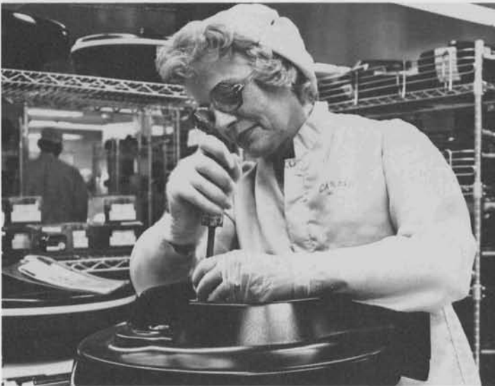
The Data Mark data module, for use with the Memorex 3640 and comparable disc drives, is assembled and sealed in clean rooms of the most rigid standards.
