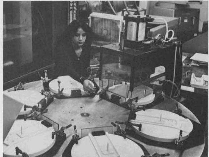
To assure that the new Mark III-F Disc Cartridge meets precise dimension standards in the manufacturing process, it is cooled after forming in this special rotating fixture.
