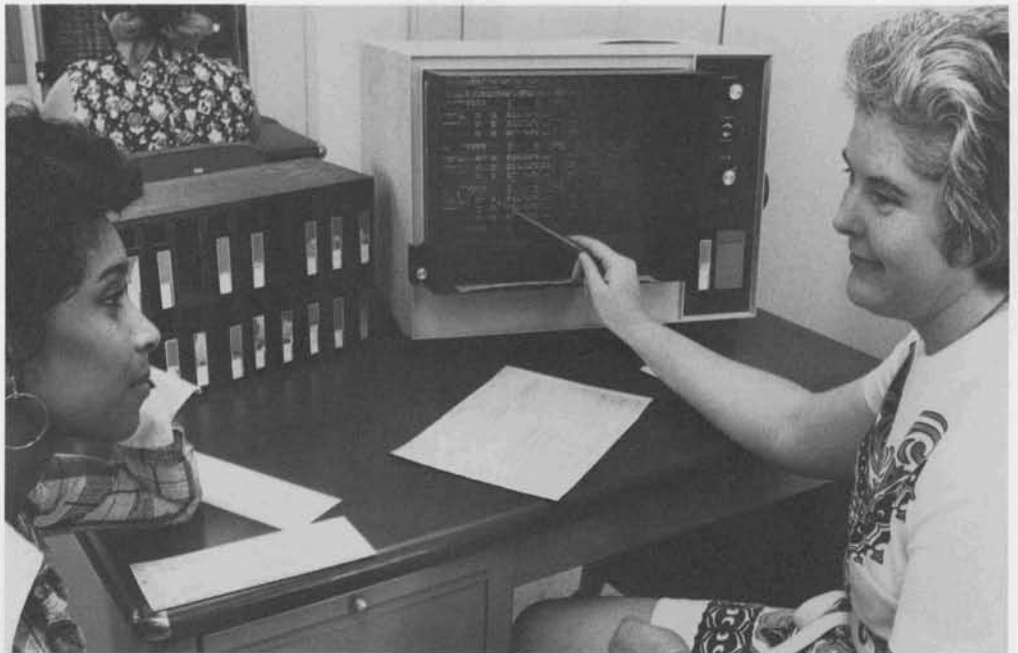
A feature of the Memorex Computer-Output-Microfilm system is the 1644 viewer, shown here at data center of the city of Richmond, Virginia. It offers rapid and easy retrieval through use of cassettes that do not require rethreading or rewinding.
