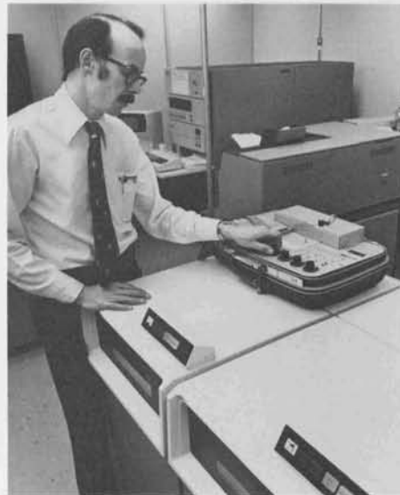
Portable diagnostic kit, providing complete testing of disc file equipment, is used by field engineer on a 3640 Disc Storage Subsystem.
