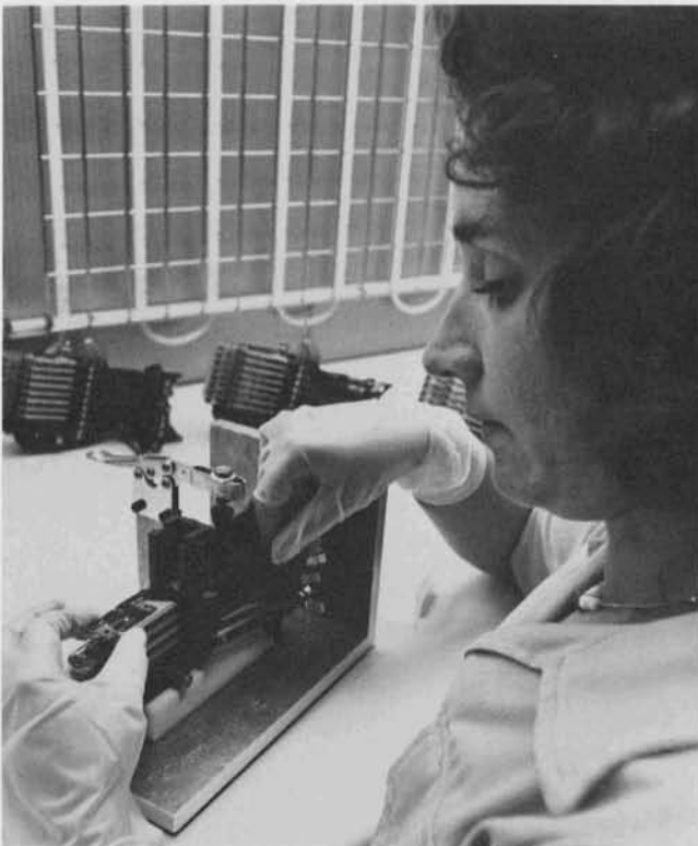
Carefully inserted in the head subassembly during the manufacturing process, the heads will record and play back information on the discs in the Head Disc Assembly of the 3650 Disc Storage Subsystem.
