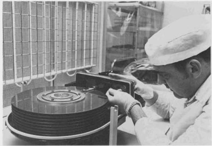
Key element in the new Memorex 3650 Disc Storage Subsystem technology is the Head Disc Assembly. It incorporates the discs (on which the information is stored) in the same unit with the read/write heads.
