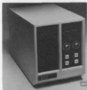
Flexible Disc Reader/Writer provides system entry to small computers. A later model will feature a keyboard and CRT.
