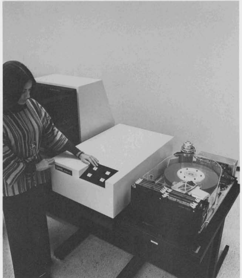
Using low mass head technology, the new 601 family of fixed disc files offers a major improvement in total system performance.
