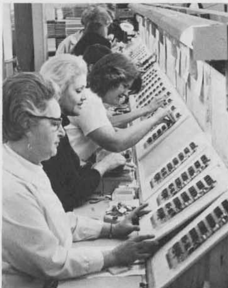
Loading electrical components into printed circuit boards along one of the PCB "speed lines" in Santa Clara are (l to r) Bertha Simas, Elsa Domingues and Mary Urista.
