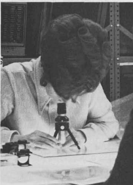
Inspecting art work for registration, line width and spacing is Sharlene Kurth. This work is done prior to printing of copies required in the production process.
