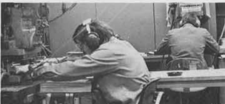
Gary Stone, of the Eau Claire Fabrication Department, utilizes a punch press for blanking circuit boards.
