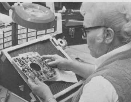
Final examination is made on a 651 Flexible Disc File Printed Circuit Board by Opal Hart, Senior Sub-assembler.
