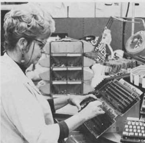
Printed circuit boards are uniquely incorporated into Memorex communication terminal key boards. Above, June Kinne, PCB Sub-assembly lead, performs final assembly work on the 1280 keyboard.
