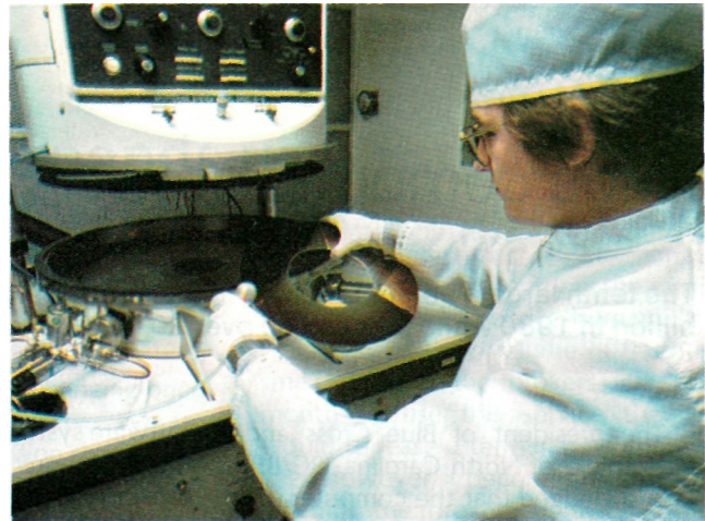
Smoother and thinner coatings of magnetic metal oxide are required for disc surfaces in order to pack more bits to the inch on high-capacity disc subsystems. Among the state-of-the-art coatings is the "M" formulation that Memorex developed.
