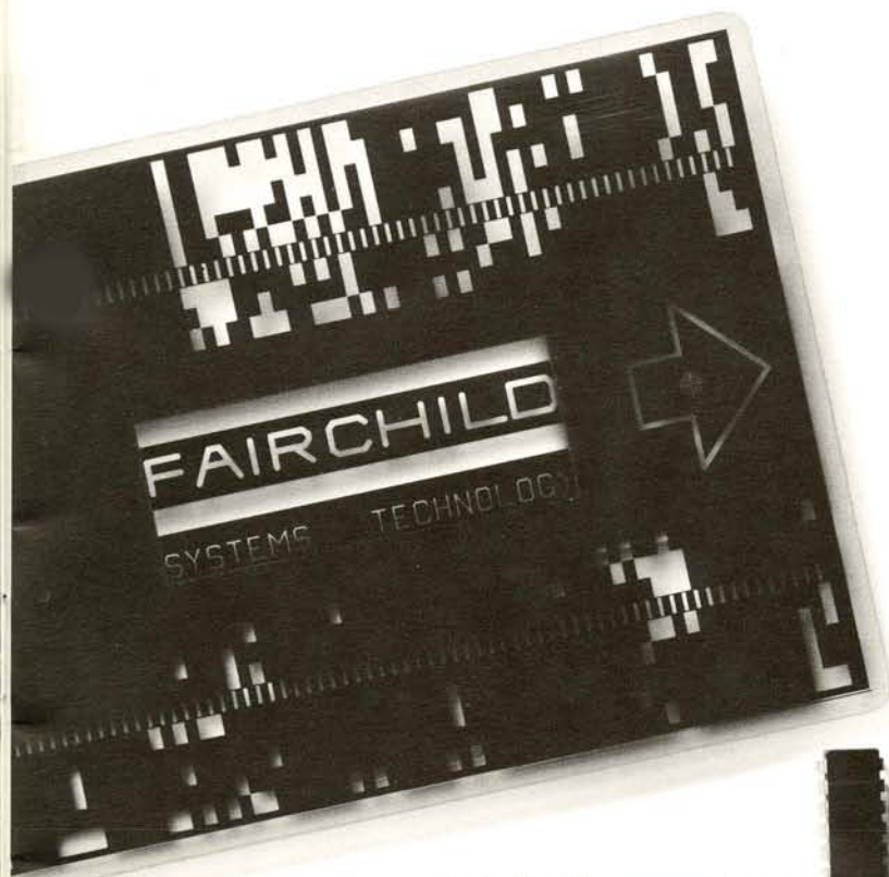
The Qualifier 901, a semiconductor test system (right) for incoming inspection by users, was introduced by the Fairchild Systems Technology Division in mid-year. The system is programmed to test a specific device with an optically coded plastic card (left).
