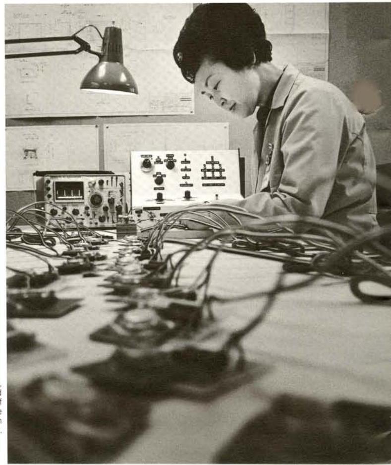
Production of solid-state ignition systems, shown during assembly, increased throughout 1974 — the first full year of operation for the company's Automotive Unit. This group supplies systems for both new cars and the replacement market.
