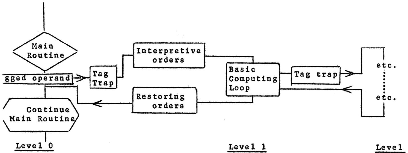
Figure 4.1.2. Relation of the Interpretive routine to the main routine and basic computing cycles.
