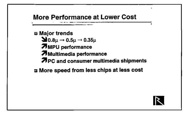
As technology is scaled, we are seeing on chip clock speeds gaining linearly, or even faster. 100 Megahertz microprocessors are becoming routine; but off chip clock speed, using traditional CMOS, IO and wide buses, things are running into some physical limits around the 66 to 80 Megahertz area.
