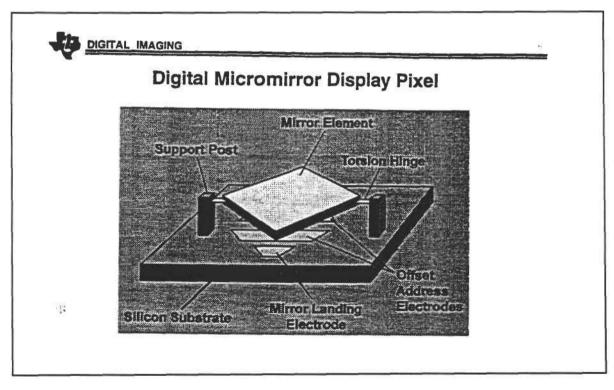
The DMD switch is approximately three orders of magnitude faster, in the neighborhood of 15 microseconds which is able to modulate light very quickly and very crisply, contributing to the resolution.
