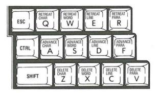
The cursor control keys permit you to move the cursor forward or backward by character, word, line or paragraph. In addition, the bottom row of keys control the erasure of characters, words, etc. as shown in the above illustration. Notice that the keys are arranged in a matrix with each row performing one of the three cursor movement functions. The 'columns' of keys designate the text to be acted upon, either character, word, line or paragraph.
