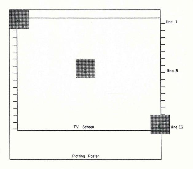
The diagram above shows the size of a single plotting square in relation to the size of the television screen and the plotting raster. By convention, the characters are plotted in the same position on the single plotting square. This allows a standard chart for base address to be used in specifying the location of the square on the television screen. The characters shown above are slightly larger than Pica type.
