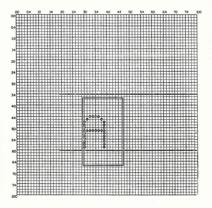
Characters to be plotted by a PLATO program are originally drawn as a series of dots (points) within a 64 x 64 point plotting square. The points which form the character are then translated into coordinate pairs which make up the bulk of a Character statement in a PLATO source program. The "A" above, in Character statement format is as follows:
