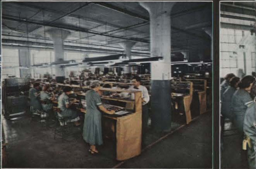
Key to serviceability of Univac is its many removable service units, known as "chassis." These are fitted into sections, three of which form each bay. Experience has proved that women are best for this precision assembly.
